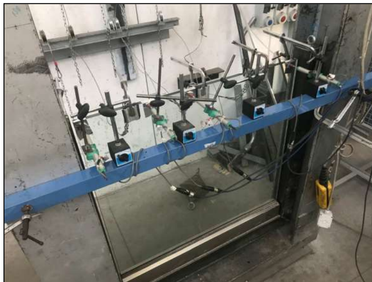
Photograph of the railing subjected to working load
